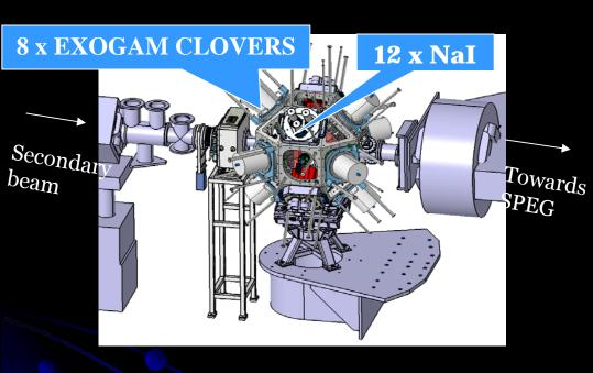
An illustration of the experimental setup at GANIL. The beam enters from the left where it interacts with the target surrounded by 8 Ge and 12 Nal detectors.
