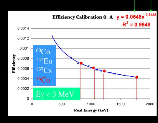
**Above:** An efficiency calibration for one of the EXOGAM clovers. *Without 56Co we cannot extrapolate the analytical expression for the efficiency beyond 2 MeV.*
